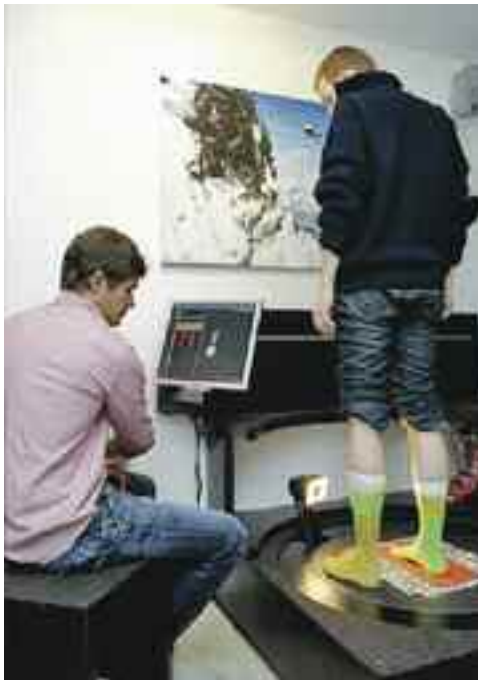
Fig. 1 Patient standing on a code marked platform with built-in pressure sensors.
